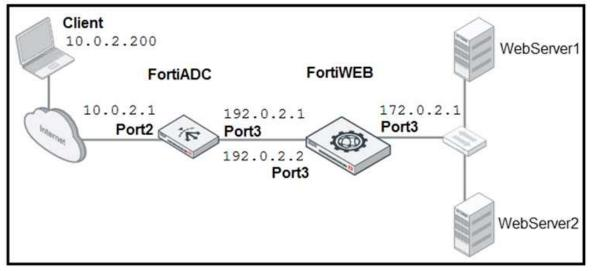
FortiADC is applying SNAT to all inbound traffic going to the servers. When an attack occurs, FortiWeb blocks traffic based on the 192.0.2.1 source IP address, which belongs to FortiADC. The setup is breaking all connectivity and genuine clients are not able to access the servers.
