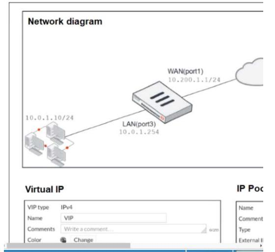
The exhibit contains a network diagram, virtual IP, IP pool, and firewall policies configuration. The WAN (port1) interface has the IP address 10.200.1.1/24.
