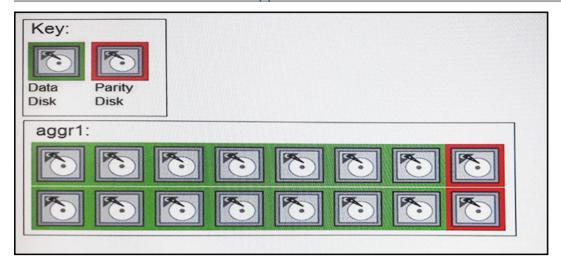
The maximum RAID group size of the RAID-DP aggr1 shown in the exhibit is 18. You expand the aggregate by 20 disks.
