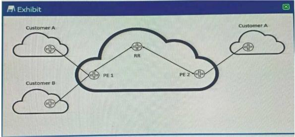
Referring to the exhibit, you want to reduce the CPU processing load on PE 2 by preventing the receipt of routes belonging to Customer B.
