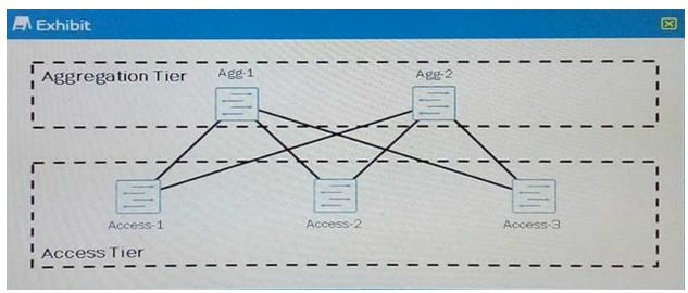
Referring to the exhibit, you are designing a Layer 2 data center and you want to make sure that all the links between the access tier and the aggregation tier are used.
