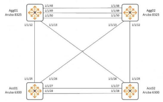
An engineer has attempted to configure two pairs of switches in the referenced configuration it is required to implement VSX keep-alive at the aggregation layer.
