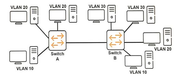
The network consists of two ArubaOS switches with routing disabled.
