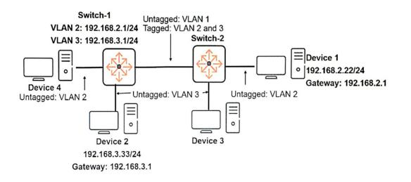
Device 1 needs to send traffic to Device 2, and it sends an ARP request in preparation.
