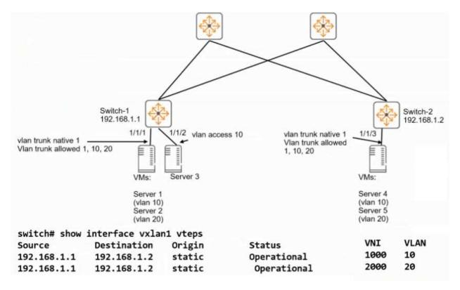
Switch-1 and Switch-2 ate ArubaOS-CX switches that implement VXLAN WITHOUT Ethernet VPN (EVPN). Switch-2 uses the same VNI-to-VLAN mappings as Switch-1. Is this how the specified servers communicate?
