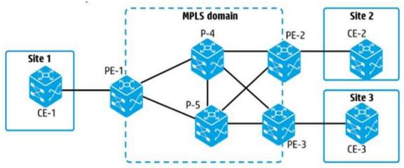
An MPLS VPLS solution (non-hierarchical) will connect the sites shown in the exhibit Which pseudo wire (PW) connections must the administrator configure?
