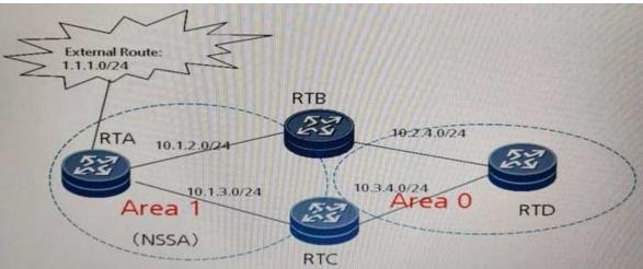
As shown in the figure, external route 1.1.1.0/24 is imported to RTA that is located in the NSSA area RTD is a backbone area router. RTB and RTC are both area border router (ABRs). OSPF configuration are as follows.
