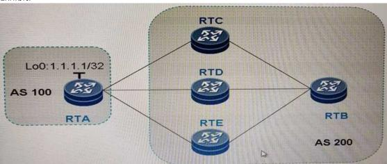
As shown in the figure, RTA belongs to AS 100 and has an EBGP neighbor relationship with RTC, RTD, and TTB is an IBGP neighbor of RTC, RTD, and RTE, and the four router all belong to AS 200.
