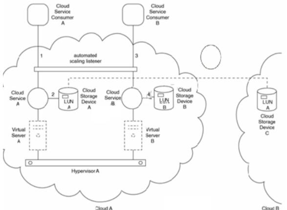
Cloud Service Consumer A issues a request to Cloud Service A (1). To process the request, Cloud Service A accesses LUN Aon Cloud Storage Device A (2). Cloud Service Consumer B issues a request to Cloud Service B (3). To process the request, Cloud Service B accesses LUN B on Cloud Storage Device B (4).
