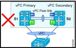
Customer has a pair of Cisco Nexus7010s switches and connected to a single Cisco Nexus5548 switch via vPC. Customer has a combination of M1 and F1 I/O Modules in Cisco Nexus7010s. Why is the design described not supported?
