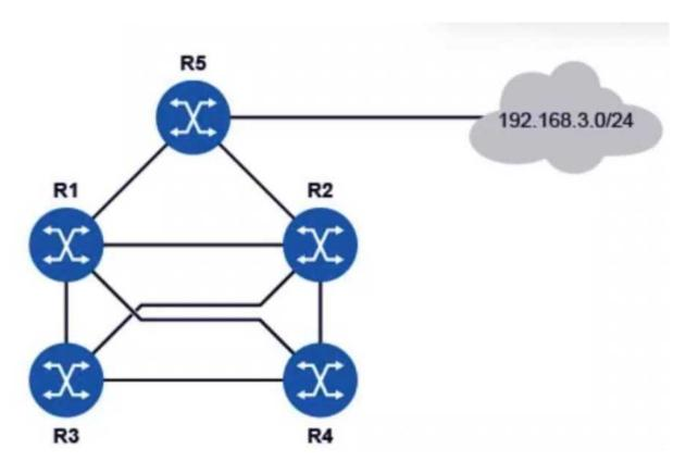
All routers in the diagram are running an interior gateway protocol (IGP) and have been configured with an ECMP value of 4. Router R5 advertises the prefix 192.168.3.0/24 using the IGP. Assuming all links have the same cost, how many entries for prefix 192.168.3.0/24 will be in router R3's routing table?
