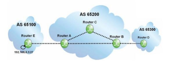
Assuming router A is configured with "next-hop-self", what does the BGP update for prefix 192.168.0.1/27 contain when it arrives at router B?
