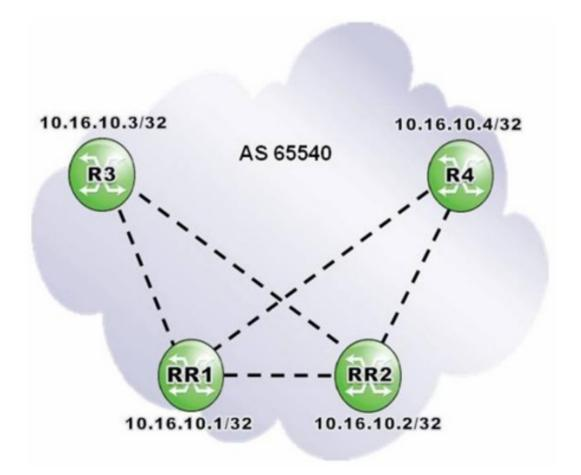
Routers RR1 are RR2 are redundant route reflectors for clients R3 and R4. Which of the following is a valid configuration on router R3?
