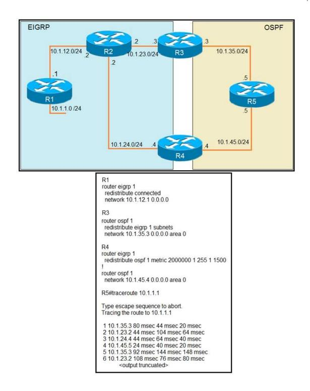
The output of the trace route from R5 shows a loop in the network. Which configuration
