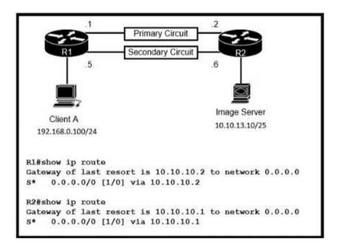
Refer to the exhibit Routers R1 and R2 have been configured with their respective LAN interfaces The two circuits are operational and reachable across WAN Which command set establishes failover redundancy if the primary circuit goes down?
