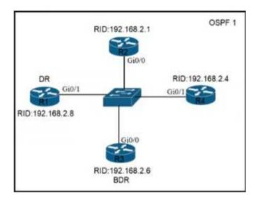
Refer to the exhibit. All routers in the network are configured R2 must be the DR. After the engineer connected the devices, R1 was elected as the DR. Which command sequence must be configure on R2 to Be elected as the DR in the network?
